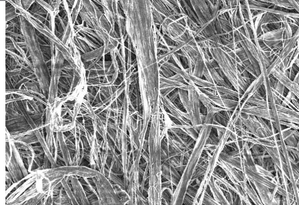
DuPont™ Tyvek® is made with a unique flash-spinning process that creates a tortuous path for particles. Image shown at 200x magnification.
